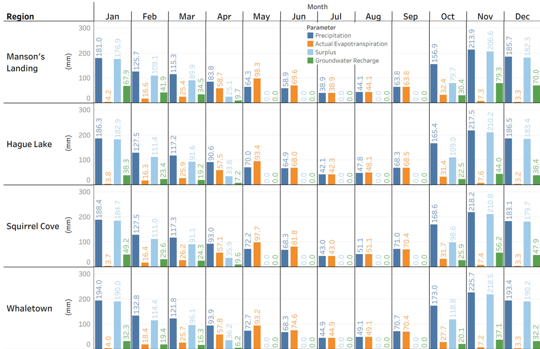
Figure 29. Water balance model results: monthly precipitation, actual evapotranspiration, surplus and recharge for Manson's Landing, Hague Lake, Squirrel Cove, Whaletown Water Management Areas.
